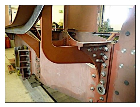
The two photos are of the new build construction of an LNER Gresley P2 2-8-2 locomotive in 12" to the foot, taking shape at the Hopetown Works, Darlington. Of particular importance is the smokebox being erected on the frames for the first time, being sponsored by the Gresley Society. Nice detail shot of the rear frames for anybody (i.e. me) building a Gresley engine with same style of foot plating, boiler and cab.
